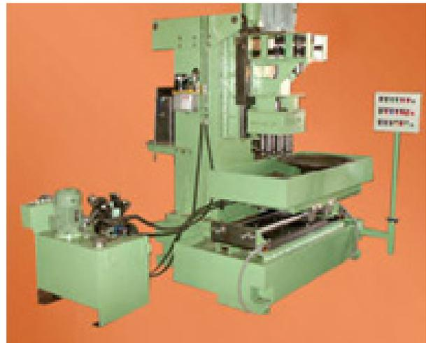
Figure 8: A special purpose drilling machine
