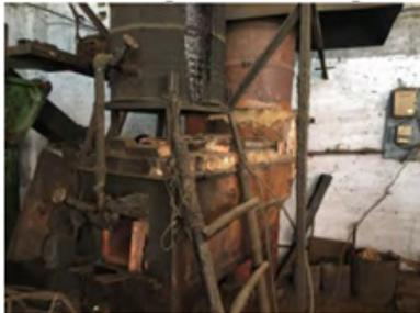
**Figure 12: An oil fired forging furnace** locally manufactured burners which are used for oil firing. Combustion air is supplied using a blower.
