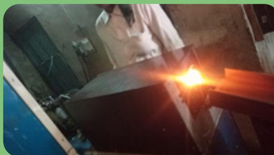
Electric Induction Billet Heater at Kohinoor Forging
